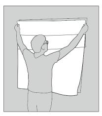
Align the Decorative Textile Film with the top of the window and press the textile gently onto the glass. Take out the remaining backing paper little by little, by section of  $\pm$  6 in each, while pressing gently the fabric onto the window from top to bottom and from the middle to the side.
