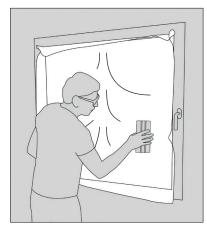
When Decorative Textile Film is perfectly flat on the window, use the squeegee to adhere it well to the glass. Press from the center outwards (see arrows). Press over the entire surface well, including the edges and the corners.
