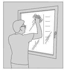
Apply a strong pressure with the squeegee over the whole Decorative textile Film surface, horizontally and vertically, in order to activate the glue. This is very important to avoid the formation of bubbles in Decorative Textile Film
