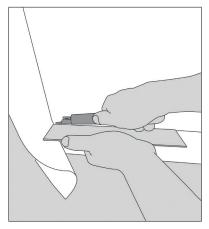
Place the squeegee next to the window silicon joint, with the cutter on the inside. Carefully cut to remove the excess, with a regular movement using strong pressure and a sharp angle. Use a new blade every 78 in and for every corner, in order to avoid tearing the yarn.
