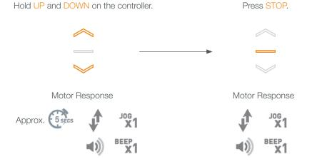
If motor is in Step Mode, use following steps to change to Roller Mode.
