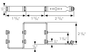
1 3/8" R-TEC Motorized Metal Traverse ONLY Pinch Pleat Master Carrier Arm, One-Way Draw Right - RTPTH138PPOR or Left - RTPTH138PPOL
