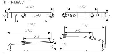
1 %" R-TEC Motorized Metal Traverse ONLY Ripplefold Butt Master Carrier Arm, One-Way Draw Right - RTPTH1380BR or Left - RTPTH1380BL
