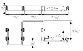
1 3/8" R-TEC Motorized Metal Traverse ONLY Pinch Pleat Master Carrier Arm, One-Way Draw Right - RTPTH138PPOR or Left - RTPTH138PPOL
