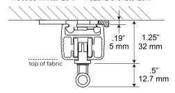
IMPORTANT: Drapery workroom must apply specific snap tape to drapery panel when using Ripplefold glides. Somfy Glydea® Ripplefold glides are only compatible with Kirsch Ripplefold snap tape. Other brand tapes are NOT COMPATIBLE with the Somfy Glydea® Motorized system.
