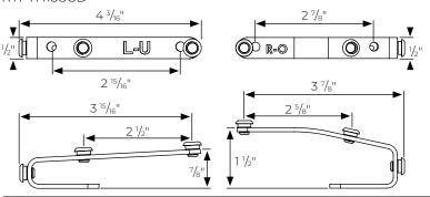
1 %" R-TEC Motorized Metal Traverse ONLY Ripplefold Butt Master Carrier Arm, One-Way Draw Right - RTPTH1380BR or Left - RTPTH1380BL
